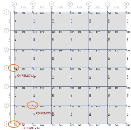
Fig.3. Column Removal Position
