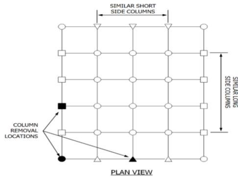
Fig.1. Location of External Column Removal
