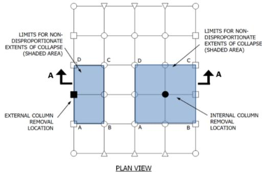
Fig.2. Allowable Extents of Collapse for Interior and Exterior Column Removal in Plan
